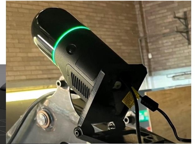
Leica Lidar scanner mounted in an optimised position on the robot system
